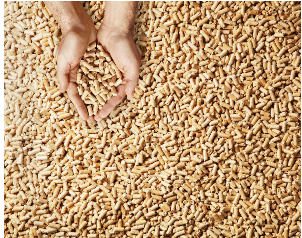
Wood pellets that replace fossil fuels in NCC's asphalt production, which results in a strong carbon dioxide-reduced manufacturing process.
